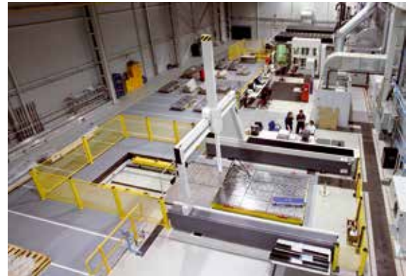
LK V-R twin-rail mounted bridge style CMM
